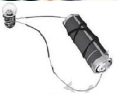
**Answer:** No, the bulb will not glow because the wires from both terminals of the battery are connected to the one terminal of the bulb. In order to make the bulb glow, wires should be connected to the both terminals of the bulb.
