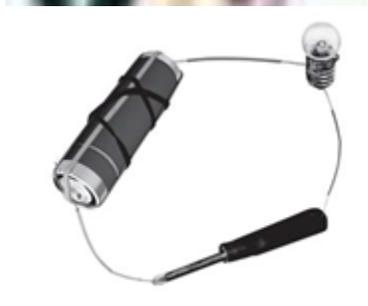
**Answer:** Bulb will not glow in the arrangement because the holder of the tester used in the connection is made of plastic which is an insulator. Thus, current will not flow in the circuit.
